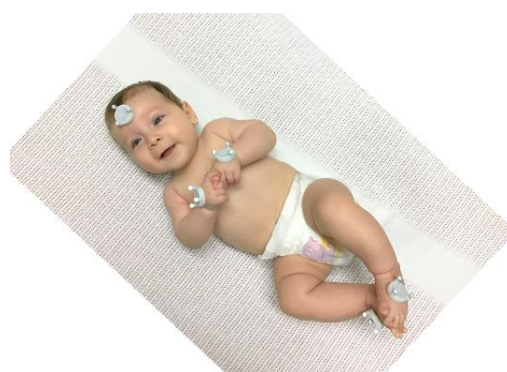
A wearable motion sensor used to measure infant movements that may help augment existing clinical assessments and facilitate earlier diagnosis of CP.
